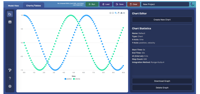
Fig. 2: Example LunaSim output showing the position and velocity of an oscillating mass-spring system over a 10-second simulation.
