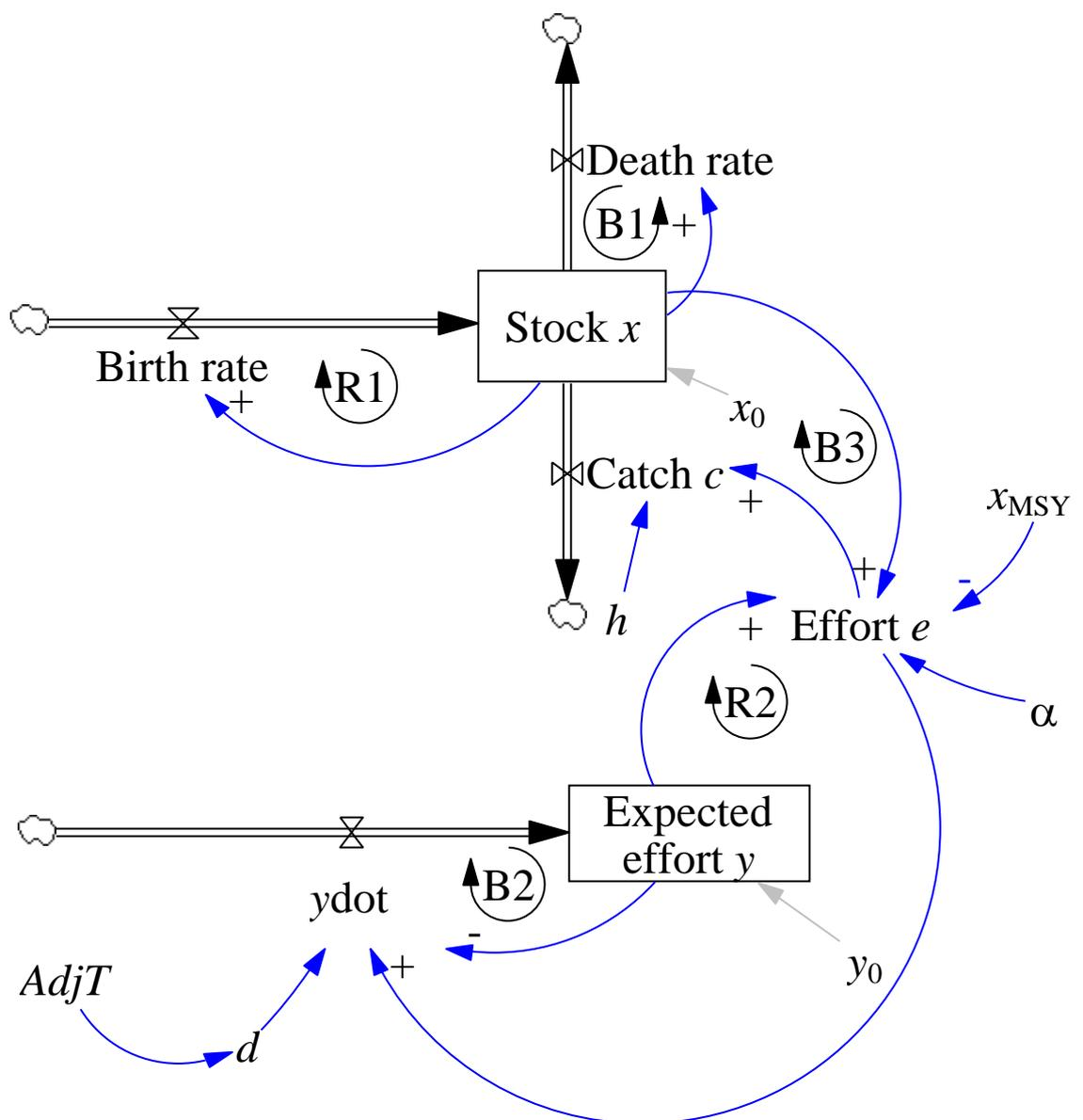
Figure 2 – The SFD of M-2 with the heuristic HCR
