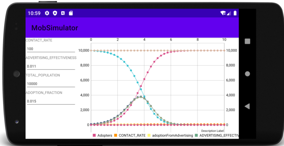
Figure 3. Mobile Simulator – automatically generated interactive simulation environment for Bass diffusion model. The interactive simulation environment is an Android mobile application. We can change model constants and re-run the simulation on a mobile phone.
