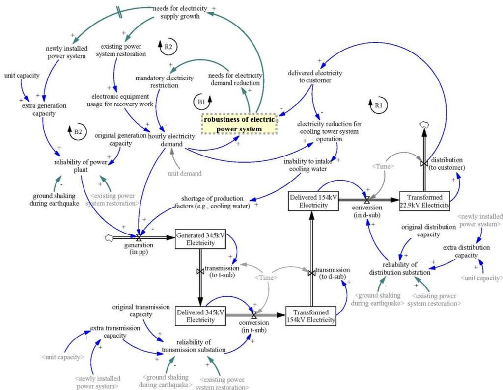
**Figure 1.** Entire model for seismic-damaged power system robustness estimation
