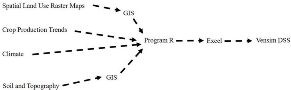
Figure 3. Conceptual diagram of processing data for Vensim™.
