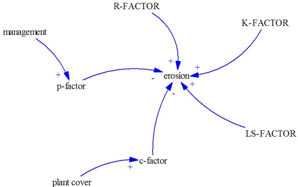
FIGURE 15. Revised Universal Soil Loss Equation integrated into the SD model and modified to capture daily cover and management impacts on aggregate rill and sheet erosion.
