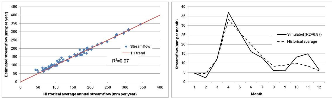
**Fig. 5.** Simulated stream flow fits well with historical records (1970s – 2000) on both spatial (left) and temporal (right) aspects.
