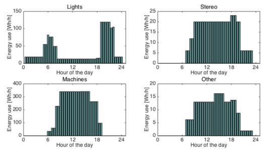
Figure 3 shows standard load profile for each of the SMEs appliances.
