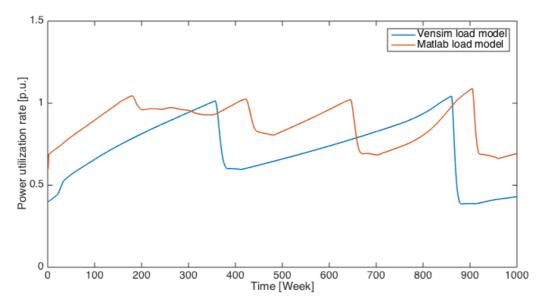
Figure 6 The graph shows power utilization rate, defined as fraction between peak power demand and installed generation capacity, for the external load model developed in MATLAB (orange graph) and the internal Vensim load model (blue graph).
