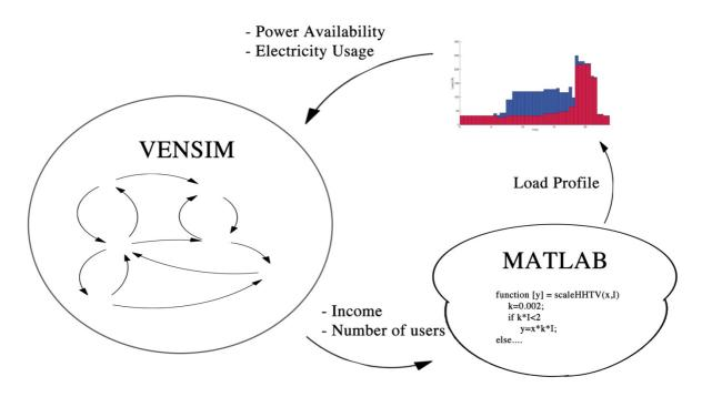
Figure 1 A conceptual diagram of the integration of Vensim with the load model in MATLAB.
