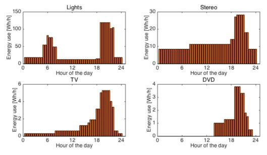
Figure 2 showing standard load profiles for each of the household appliances.
