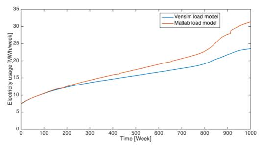
Figure 7 The graph shows total electricity usage in the minigrid for the external load model developed in MATLAB (orange graph) and the internal Vensim load model (blue graph).
