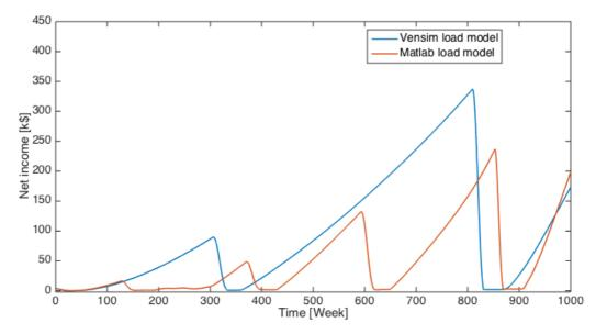
Figure 5 The graph shows the utility's financial balance using the external load model developed in MATLAB (blue graph) and the internal Vensim load model (orange).
