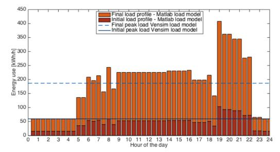
Figure 4 The graph shows initial and final load profiles using the external load model developed in MATLAB and the internal Vensim load model.
