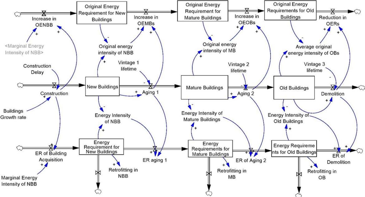
Figure 3: Stock-and-flow-diagram of the building sector
