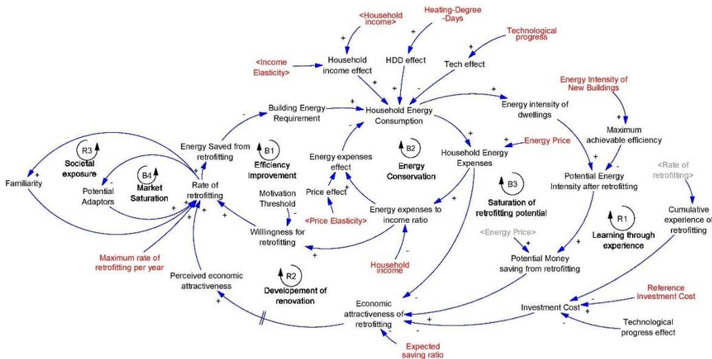
Figure 1: Causal loop diagram of energy consumption in dwellings
