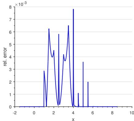
(b) Relative difference between linear and smooth interpolation of Cost of Technology Advance Table data
