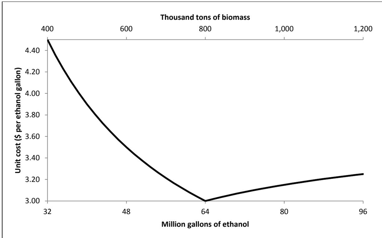
**Fig 3.** Average total production cost curve for a stylized biorefinery with feedstock throughput mapped to ethanol production.
