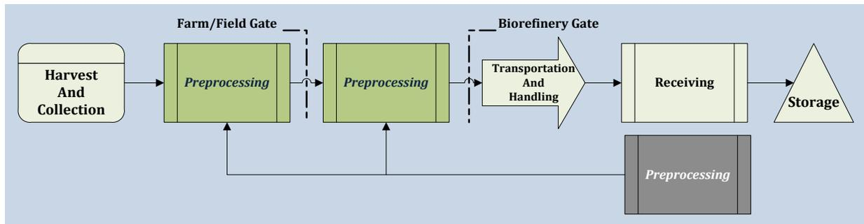
**Fig 2. Advanced supply system design (Advanced Uniform) follow the model of the current grain commodity supply system, which manages crop diversity at the point of harvest and/or depot, allowing all subsequent feedstock supply system infrastructure to be similar for all biomass resources (Argo et al., 2013).**
