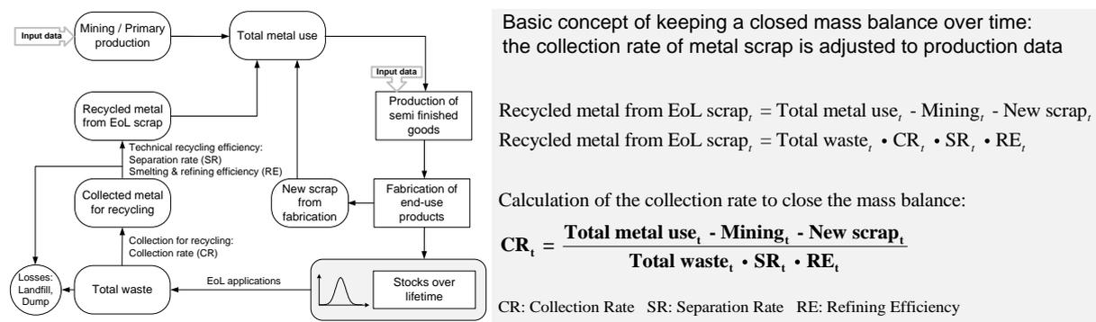
Figure 4 Enabling a closed mass balance over time by defining the global collection rate of EoL (End-of-Life) copper scrap as a function of reported global production data.
