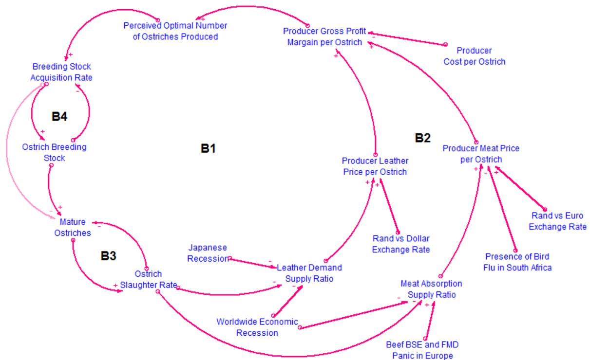
Figure 2: Aggregate causal loop diagram of system
