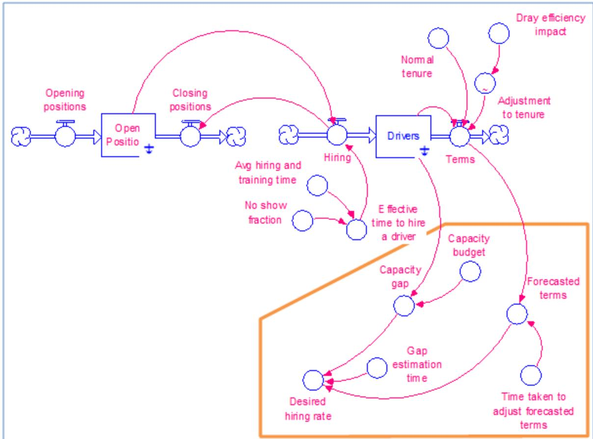
Figure 3 - Calculating the desired hiring rate
