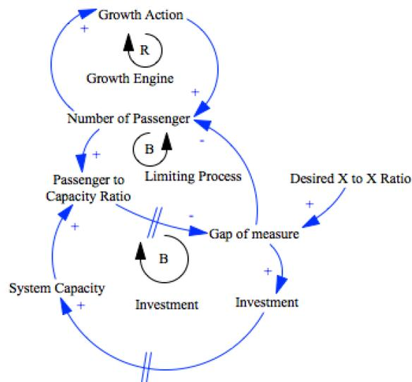
Figure 4: Causal Loop Diagram of Demand Growth, Inhibiting Process and Investment Delay forming a system archetype of “Growth and Underinvestment”.
