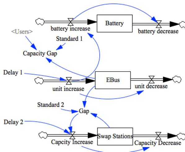
Figure 8: Co-flow of Ebus, Batteries and Swap Station as system capacity increases
