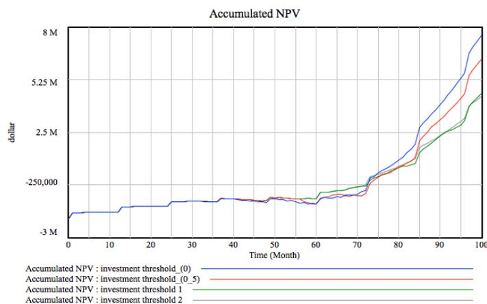
Figure 24: Net Present Value of System at various system capacity expansion sizes
