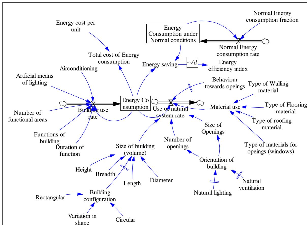
**Fig 5. System dynamic model (proposed stock flow diagram) assessing energy consumption in buildings. Please note this is only a proposed diagram there is still on-going data collection.**
