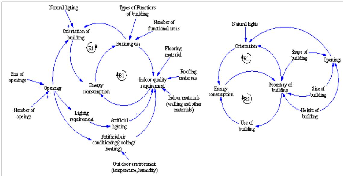
Fig 3 Causal feedback loop diagrams for energy efficiency in buildings
