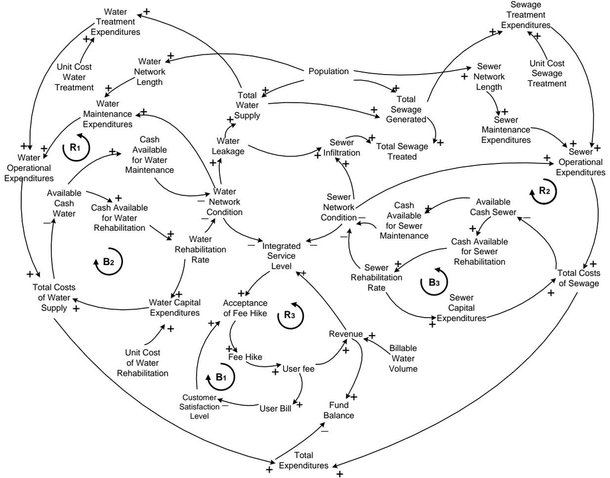
**Figure 2:** A Causal Loop Diagram for the Integrated Asset Management of Water Distribution and Wastewater Collection Networks
