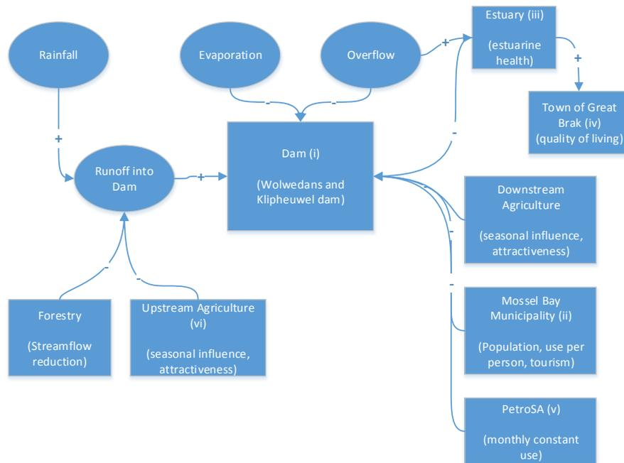
**Figure 3: Connected Sub-Models in Dam Operation Model**
