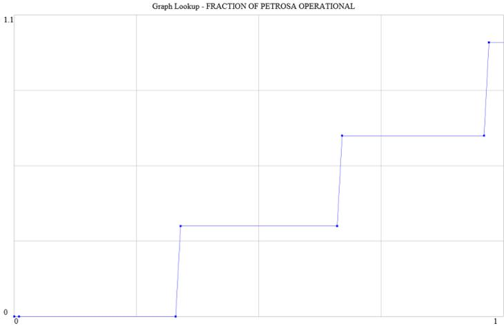
**Figure 9:** Table function for the level of operating at PetroSA depending on the fraction of demand for water supplied.
