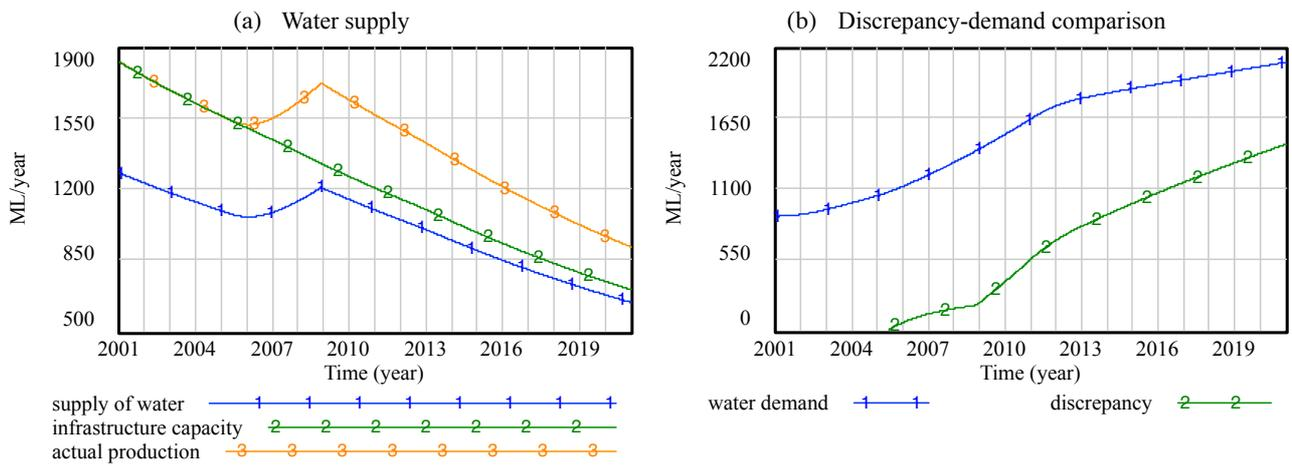
**Figure 4: The left-hand graph (a) shows the reference mode behaviour for water supply; the right-hand graph (b) compares the total water demand (line 1) to the discrepancy (line 2), which is the gap between the demand and the water delivered.**
