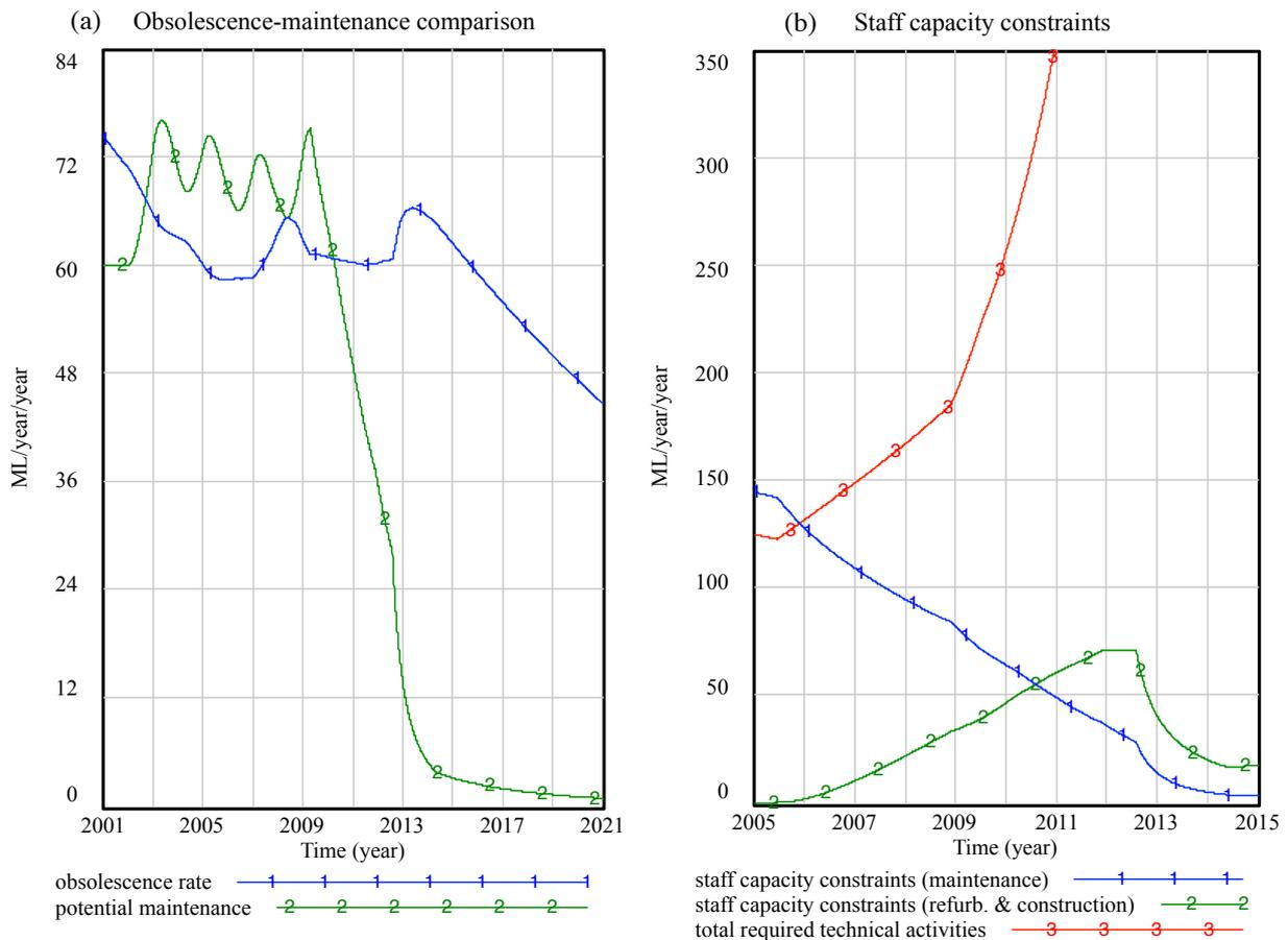
**Figure 5: Comparison of the obsolescence rate and the overall maintenance that can be performed is displayed, termed 'potential maintenance' (left-hand graph (a)); the right-hand graph (b) compares the constraints on staff capacity in the reference mode in a time segment from 2005–2015, in relation to the total required technical activities.**
