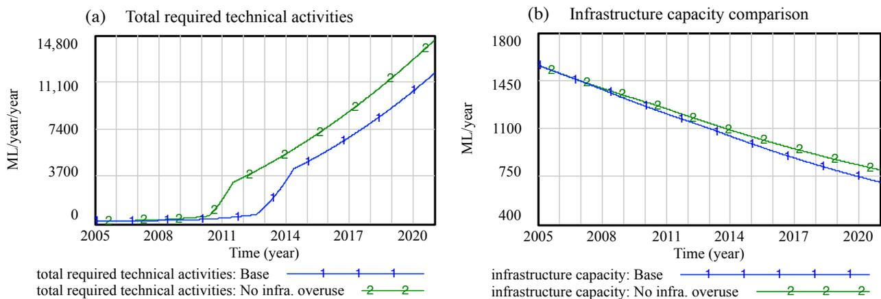
**Figure 7: Comparison of the ‘total required technical activities’ between the baseline simulation and the ‘no infrastructure overuse’ situation (a); the right-hand graph (b) compares the infrastructure capacity across the two simulations (both graphs showing a time fragment from 2005-2021).**
