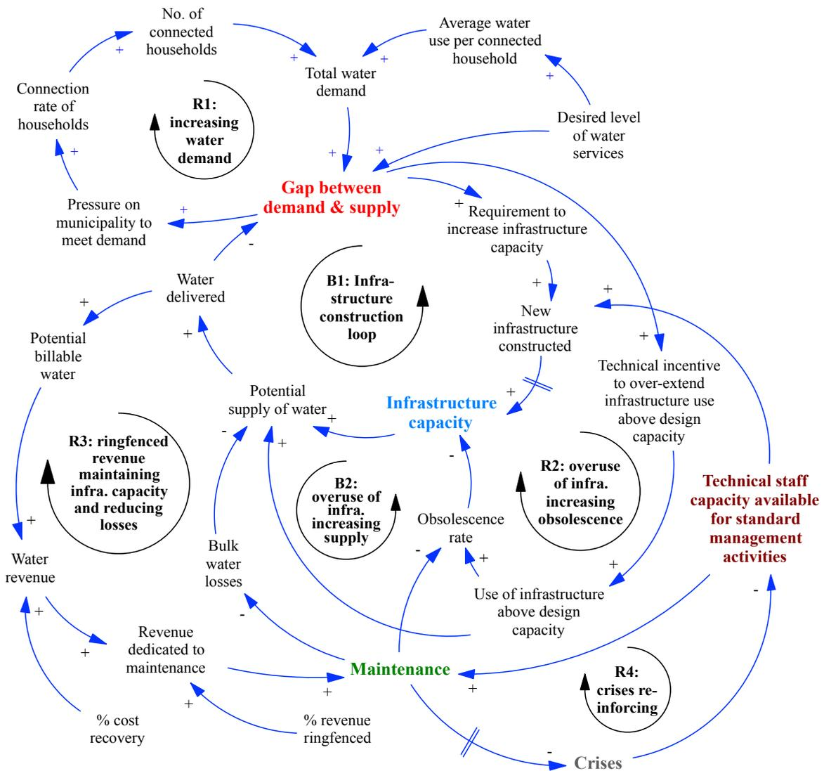
**Figure 2: Aggregate causal loop diagram (CLD) for the ‘modes of failure’ model. Six feedback loops are identified in the CLD: two balancing loops (B1 and B2); four reinforcing loops (R1, R2, R3, and R4).**
