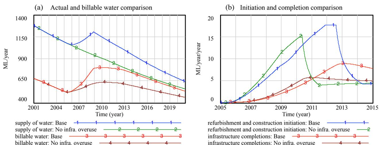
**Figure 6: Comparison of the base and ‘no infrastructure overuse’ situations: (a) compares the actual supply of water and the billable water in both situations; (b) compares the rate of ‘initiation of refurbishment and construction’ to the rate of infrastructure completion on the Greater Kirkwood water supply scheme in a time segment from 2005–2015.**
