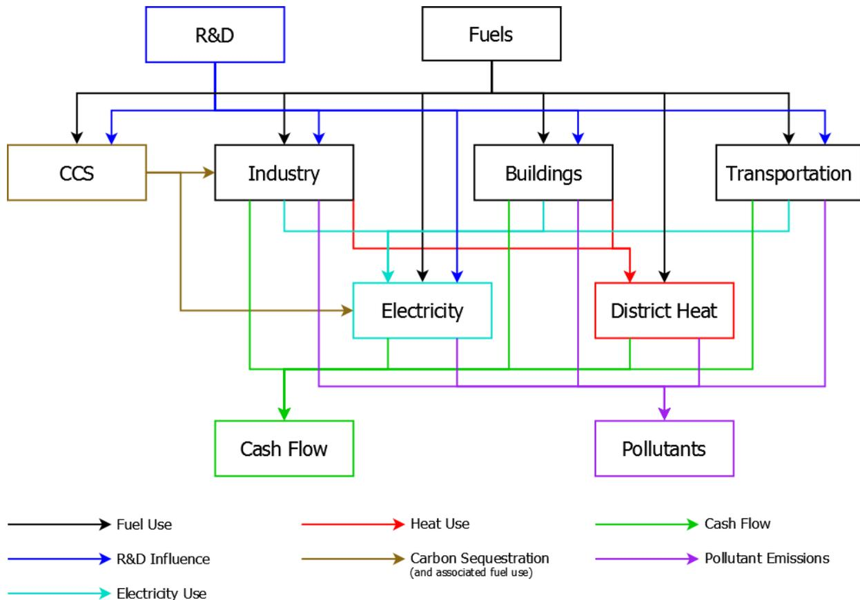
**Figure 1: Diagram of the Policy Solutions model structure**
