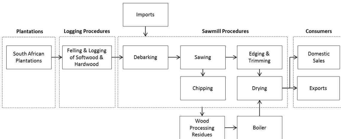
**Figure 3: System architecture map for the sawlogs product stream**
