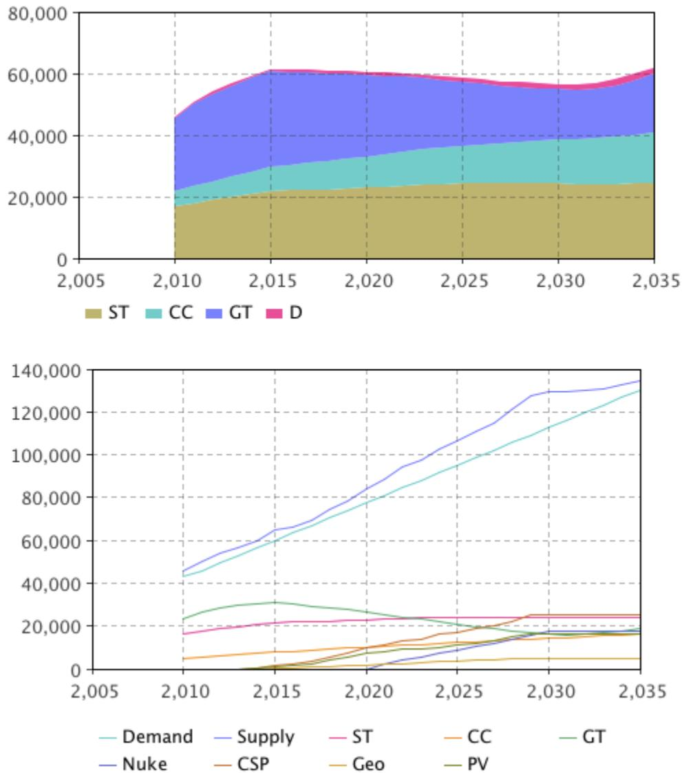
Figure 7: Top graph shows mix of conventional technology capacities over time (ST = steam turbine, CC = combined-cycle, GT = gas turbine, D = diesel generator); bottom graph shows total supply, demand, and all technology capacities over time, including alternatives (Nuke = nuclear, CSP = concentrating solar power, Geo = Geothermal, PV = photovoltaic). Both graphs are in MW.
