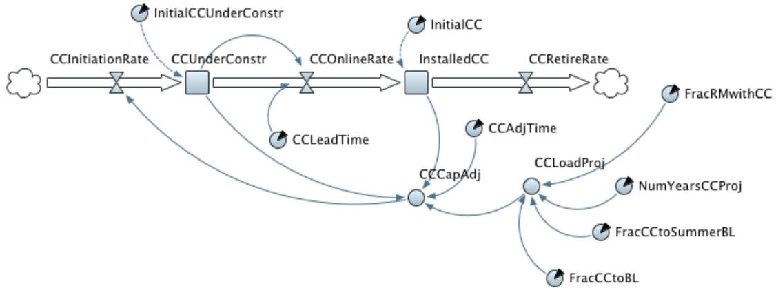
Figure 5: New additions of conventional capacity initiate according to a balancing feedback loop that seeks to close the gap between demand and alternative supply.
