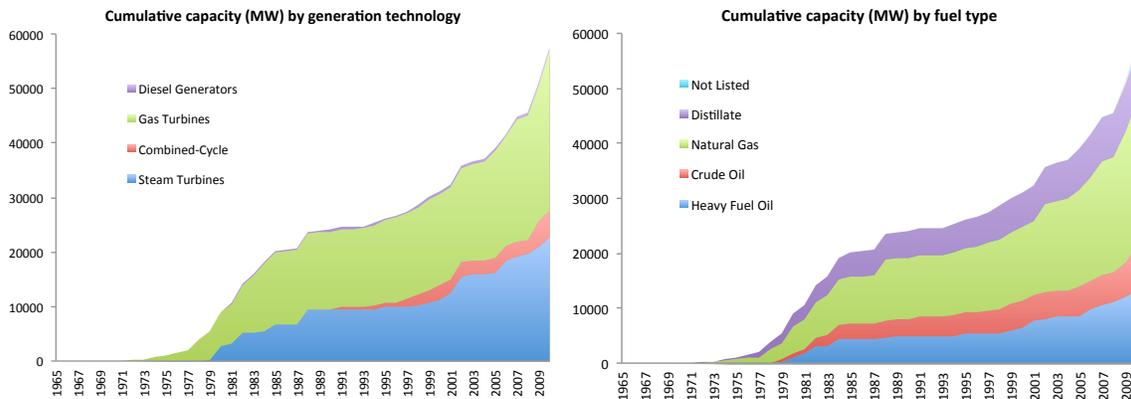
**Figure 3: KSA electricity generation is 100% thermal, consisting primarily of steam and gas (combustion) turbines fired by natural gas and various fuel oils. As can be seen from both graphs, cumulative installed capacity has grown tremendously over the past several decades. (ECRA, 2012b)**
