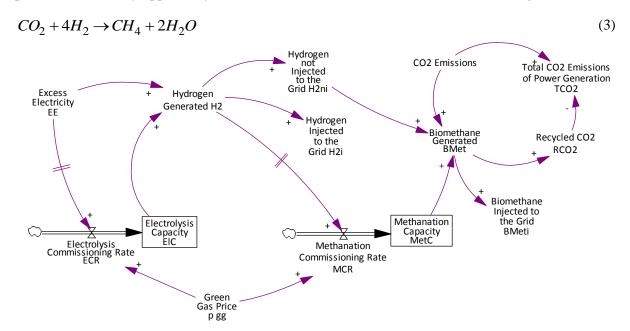
Figure 11 Stock Flow Diagram of the Power-to-Gas Sub-model
