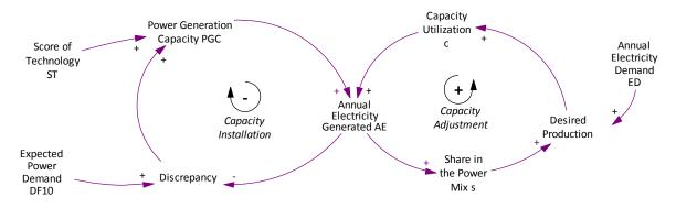
Figure 2 Causal Loop Diagram of Electricity Generation Model - Capacity
