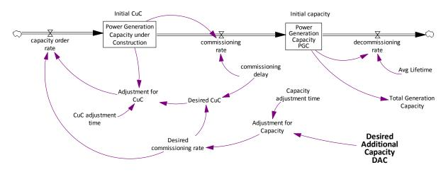
Figure 5 Stock-Flow Diagram of the Power Generation Capacity Installation
