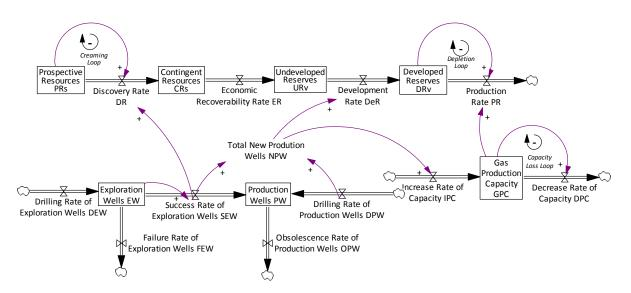
Figure 6 Stock-Flow Structure of the Natural Gas Production Sub-model
