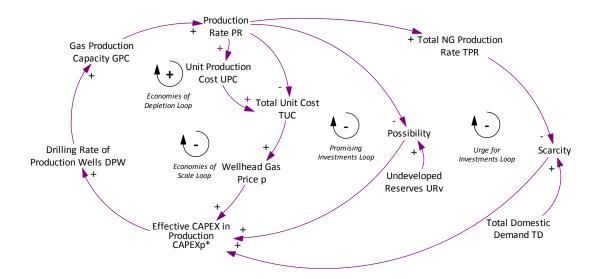
Figure 7 Causal Loop Diagram of Investment Making in the Gas Production
