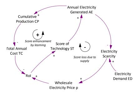
Figure 3 Causal Loop Diagram of Electricity Generation Model - RoI
