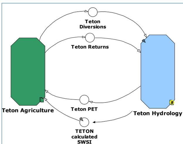
**Figure 8:** Coupling of agriculture to hydrology object
