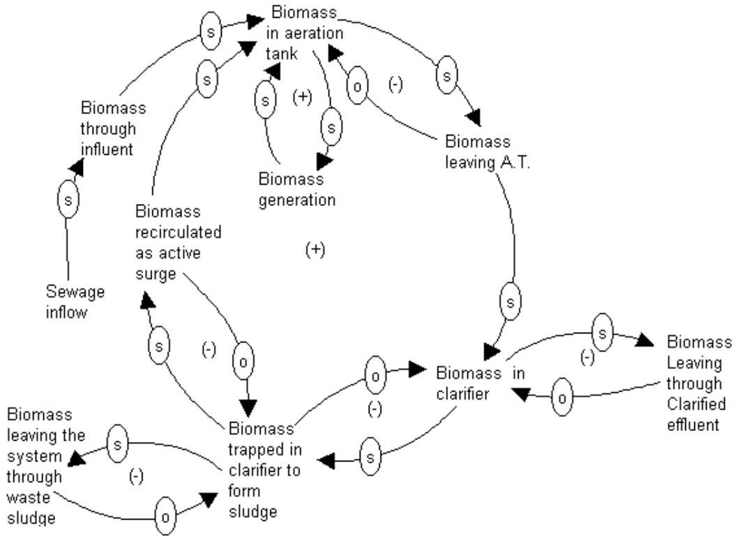
**Figure 3 Causal Loop Diagram of Biomass in Activated Sludge Treatment System**
