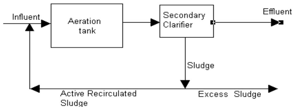
**Figure 1: Schematic Diagram of Activated Sludge Treatment System.**
