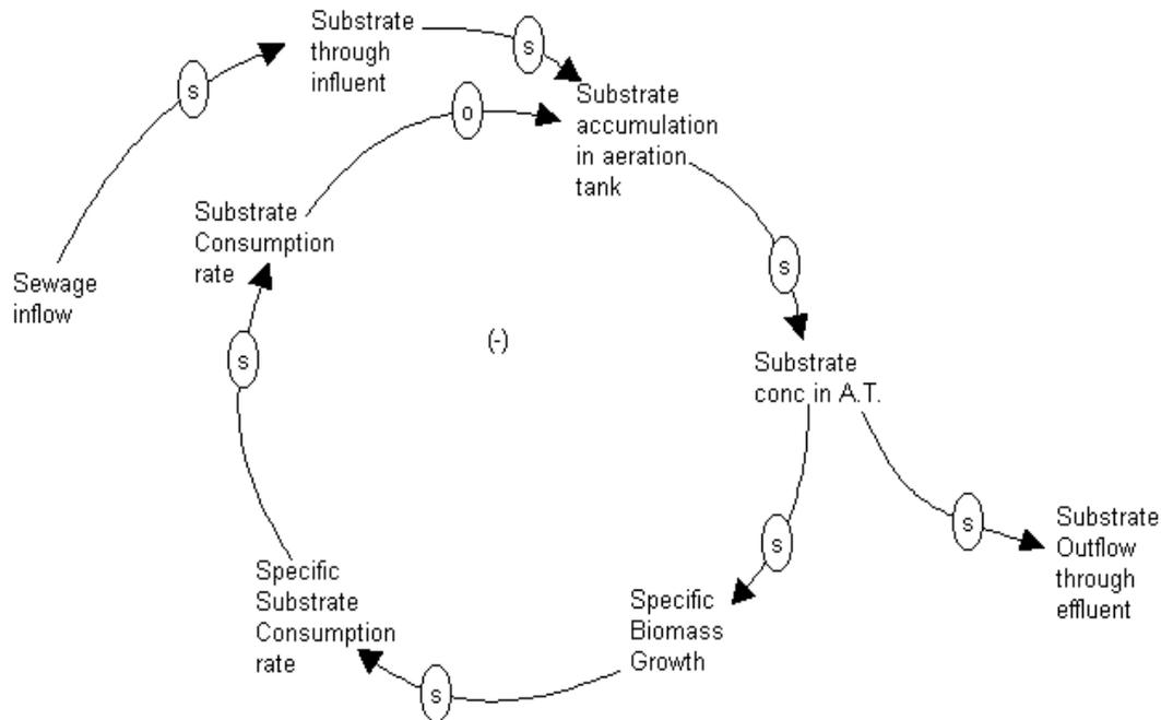
**Figure 4 Causal Loop Diagram of Substrate in Activated Sludge Treatment System**
