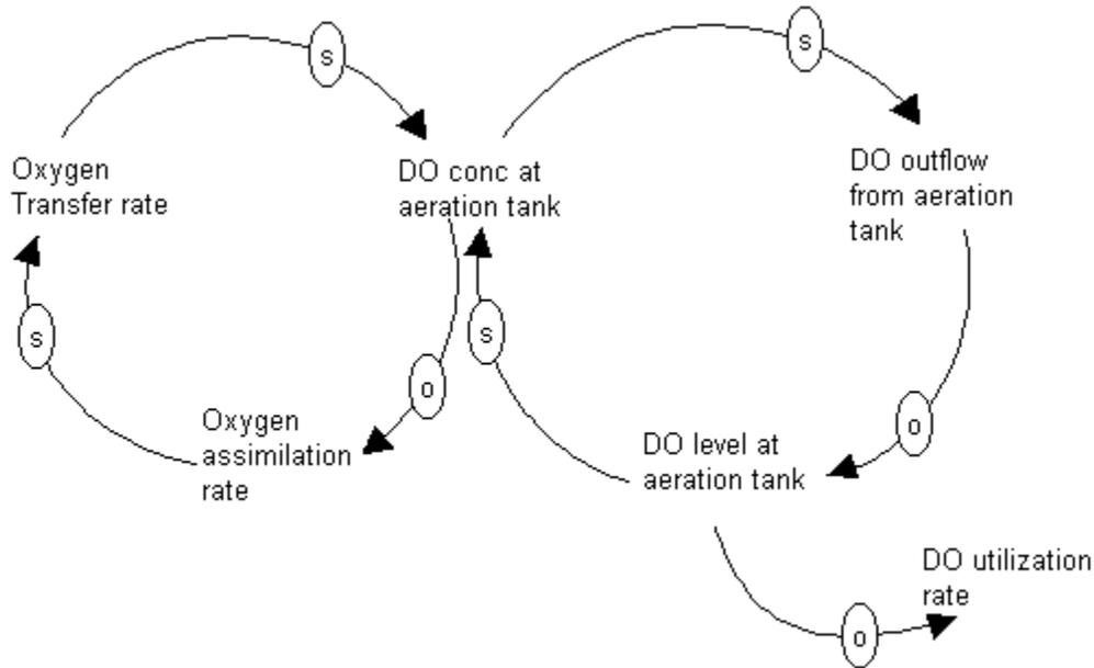
**Figure 5: Causal loop diagram of Dissolved Oxygen in Activated Sludge Treatment System**
