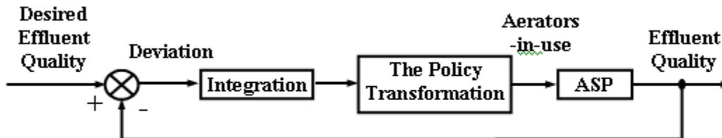
**Figure 10 Output-Integrated Feedback Control**
