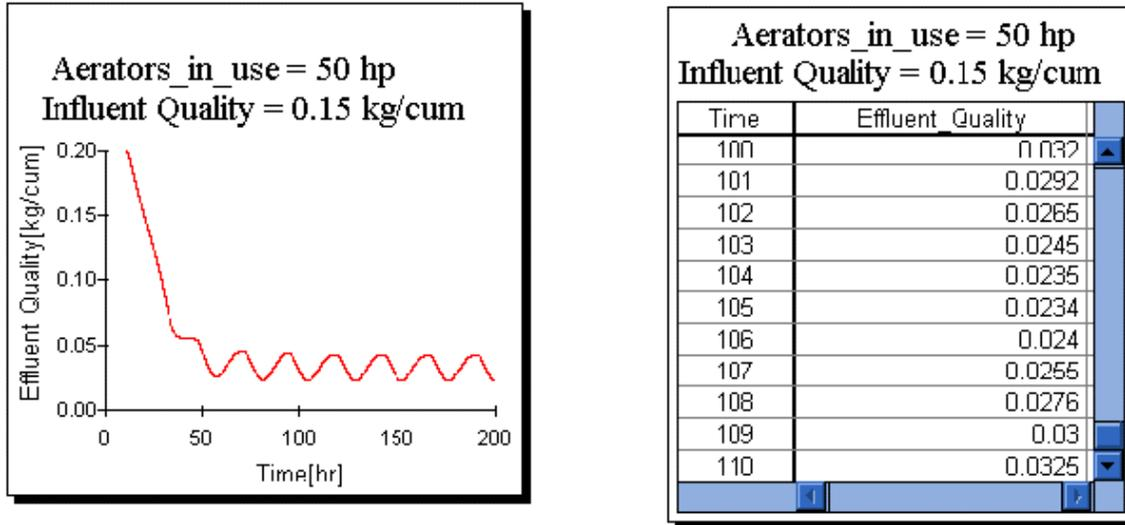
**Figure 7 Effluent Quality response for Aerators\_in\_use = 50 hp**
