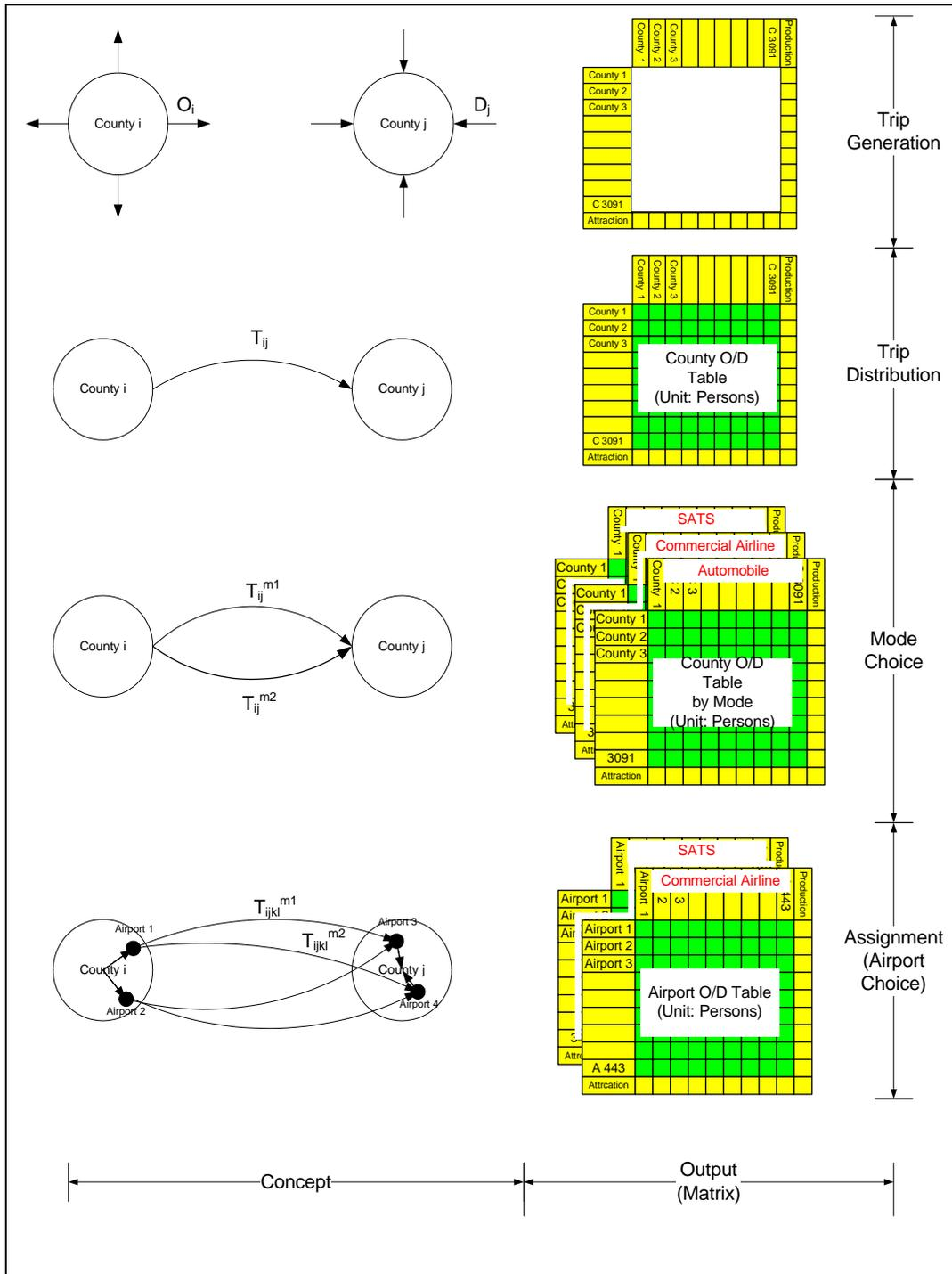
Figure 2. Multi-step Process of Trip Demand Analysis.
