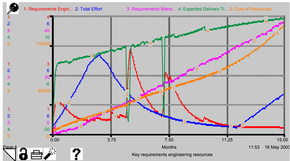
Figure 7: Simulation Output: Requirements Engineers, Cost of resources and Expected Delivery Time
