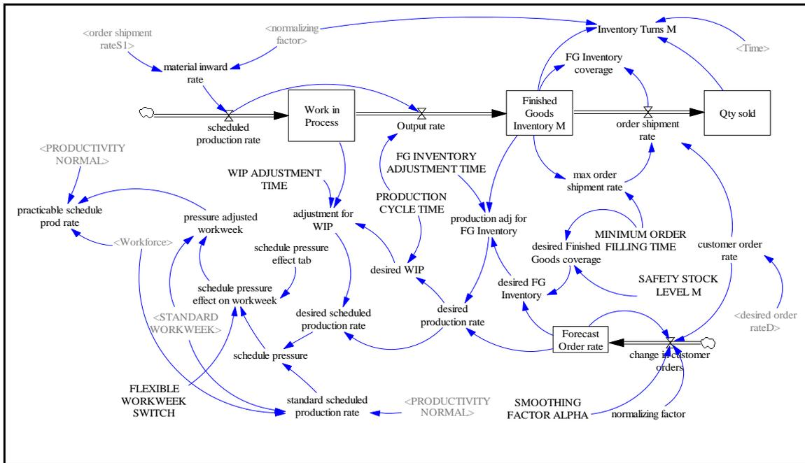
**Figure 3: Manufacturer's setup- production and inventory view.**
