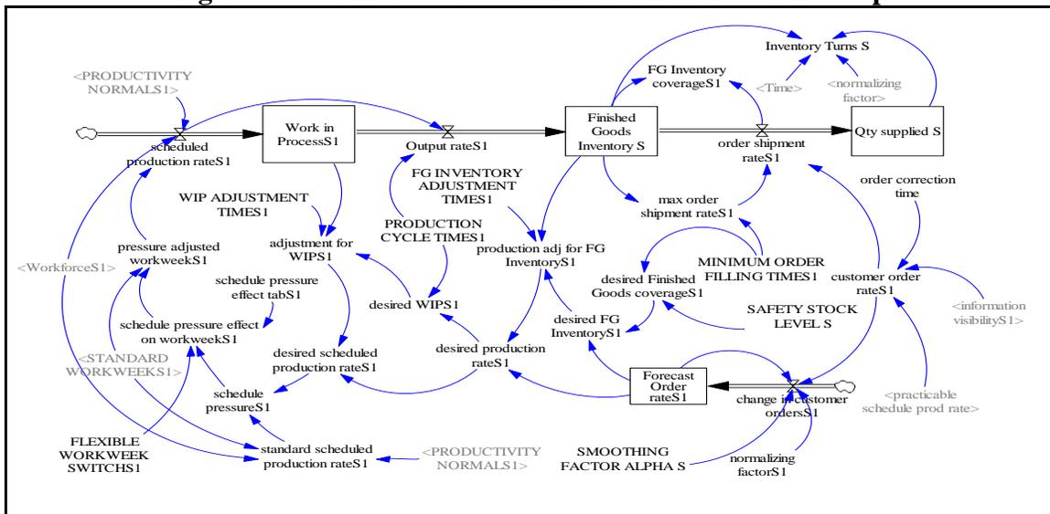
**Figure 5: Supplier's setup- production and inventory view.**
