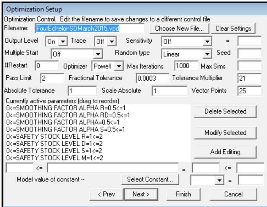
**Figure 18: Defining the search range for parameters for optimization OPT2**
