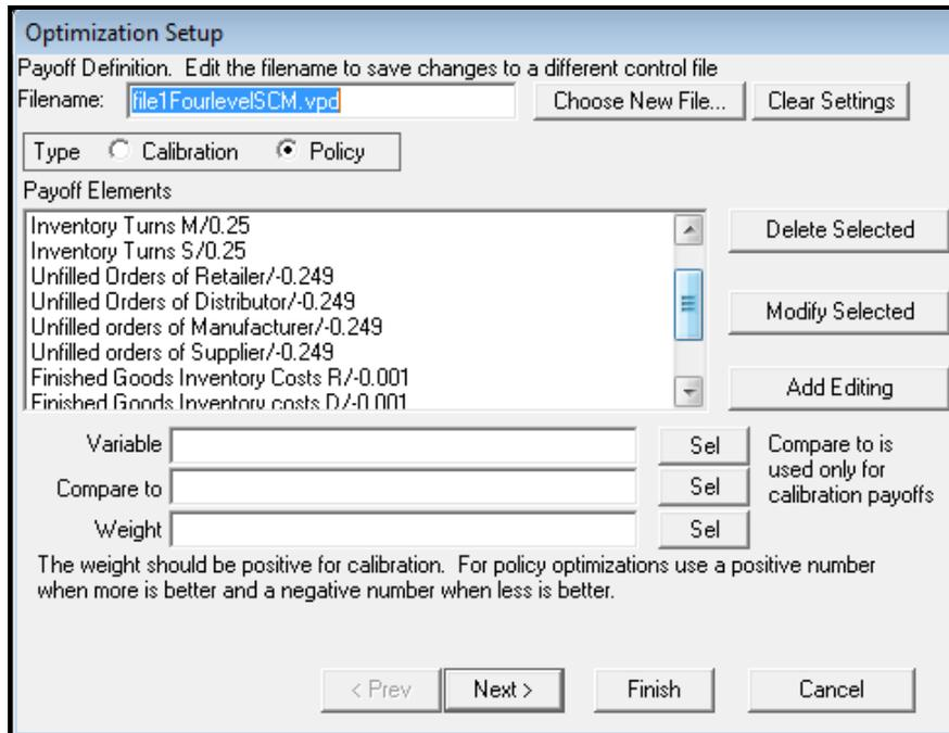
**Figure 17: Selecting the payoff elements for optimization scenario OptB**
