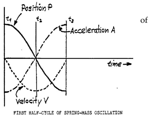
Figure 2: Explaining a Spring-Mass Cycle by its using Mass-Senge approach (from Graham, 1977, Reproduced by permission of MIT System Dynamics Group
