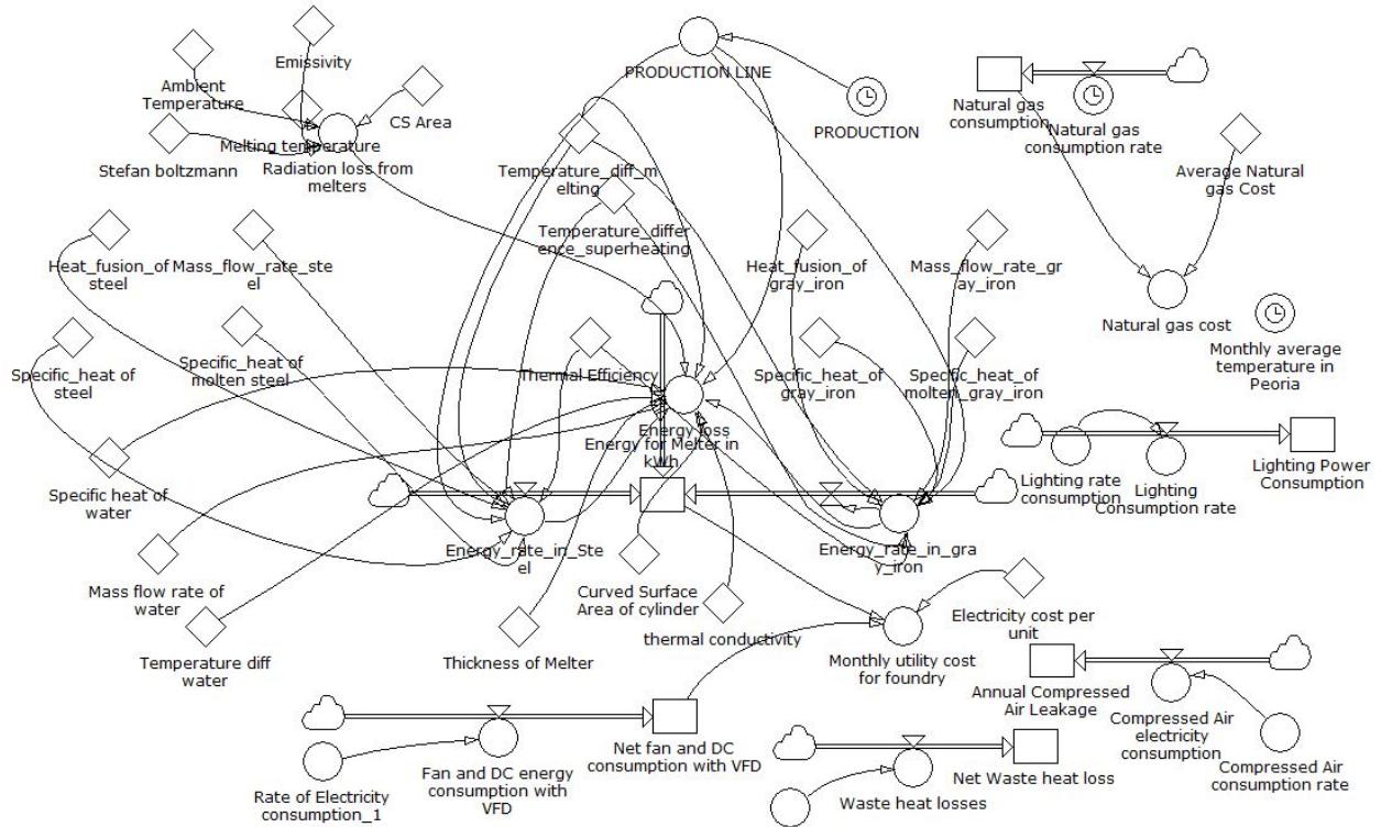
**Figure 3 Snapshot of the Powersim model**
