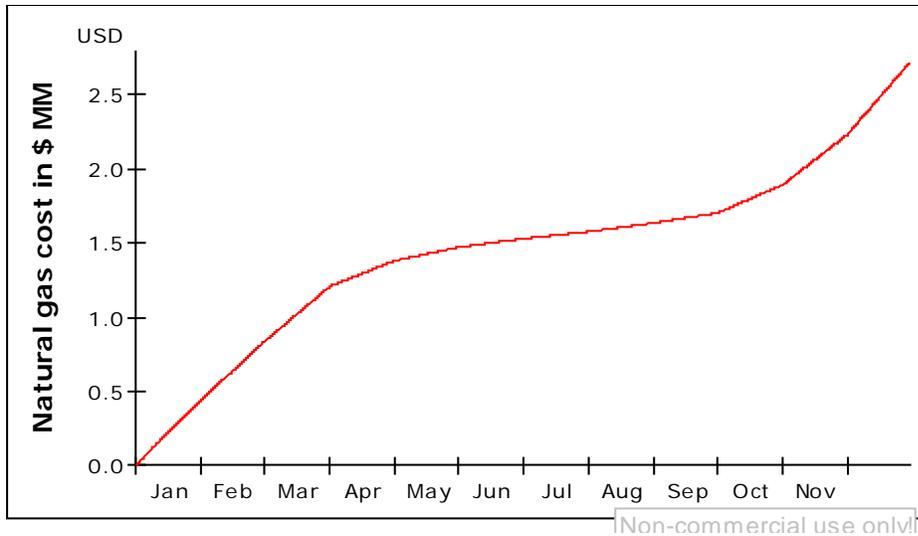
Figure 7 Actual Natural gas usage costs in the foundry during 2013-14.
