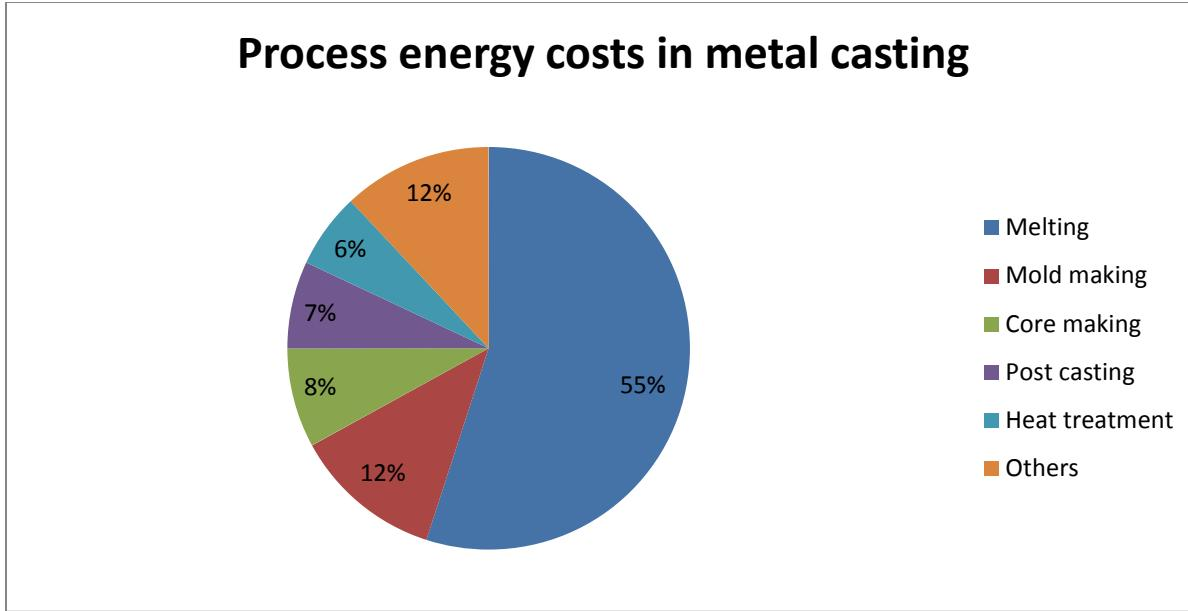
Figure 1: Process Energy costs in Metal Casting [6].
