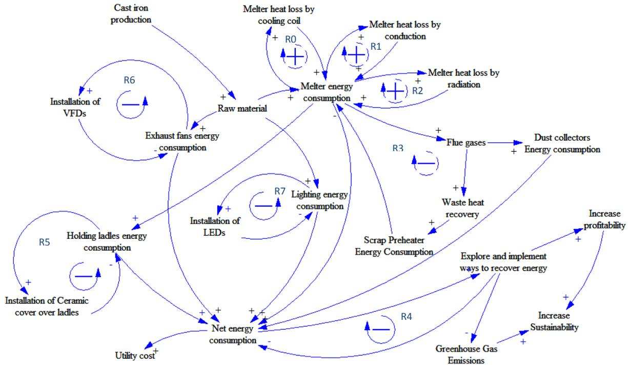
Figure 2 Causal loop diagram of energy intensive variables
