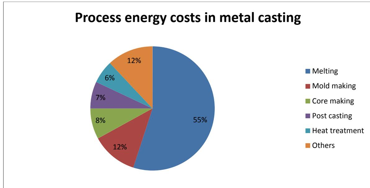
Figure 1: Process Energy costs in Metal Casting [6].
