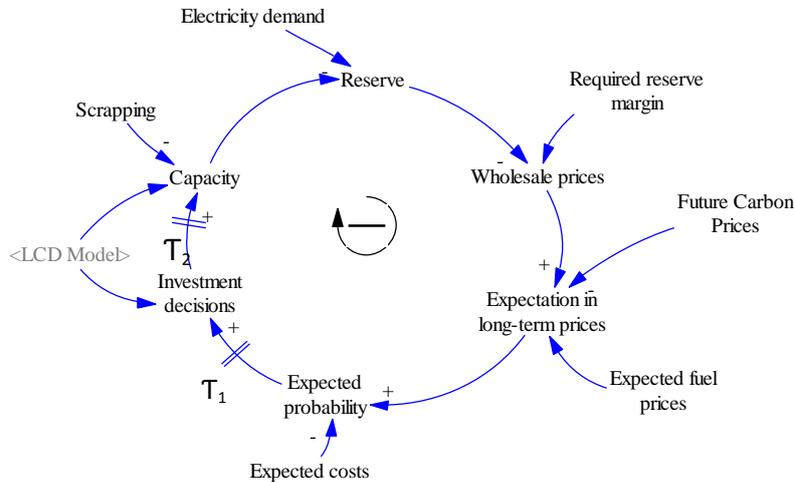
**Figure 7b** Causal-Loop Diagram (CLD) of a typical electric power system (adopted from Olsina, 2005)
