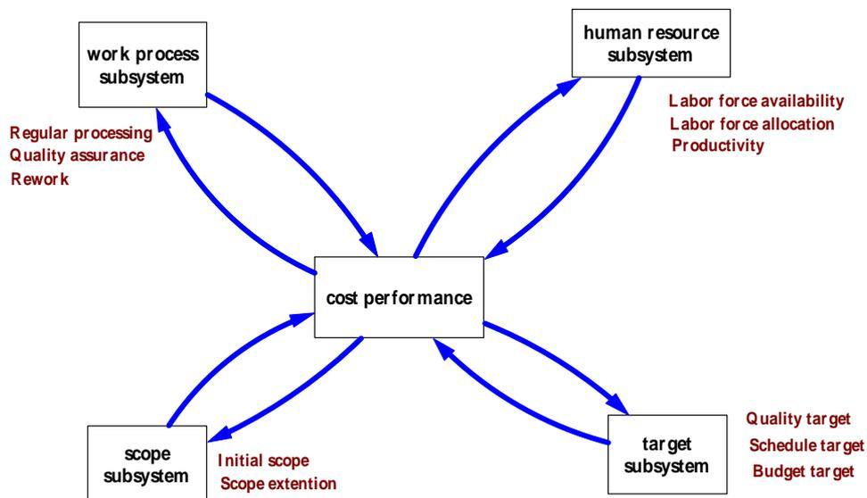
Figure 2 Interaction between subsystems in a single phase
