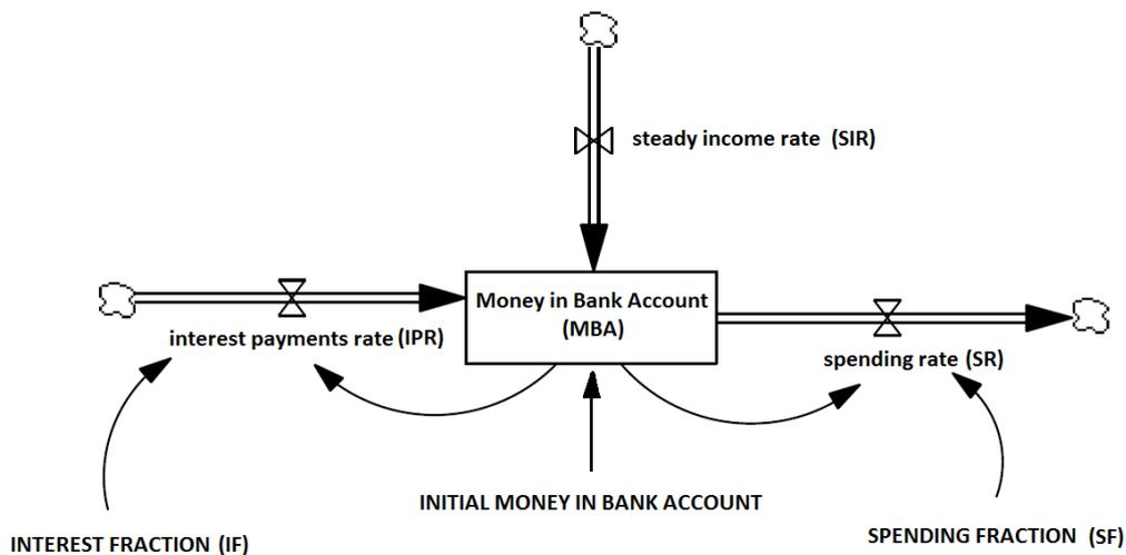
Figure 5: Bank in account model stock and flow diagram
