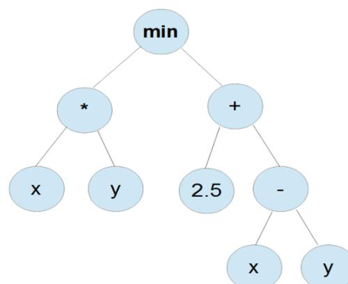
Figure 2: GP tree representing the program  $\min(x*y, 2.5+x-y)$
