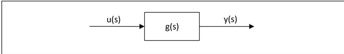
Figure A.1 The most basic block diagram representing an input-output relationship in the Laplace domain
