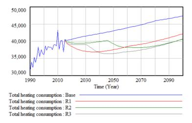
Figure 15: Comparison of total energy consumption for space heating in three retrofitting scenarios and base scenario
