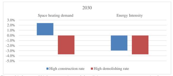
Figure 14: Impact of high construction and demolition rate on energy consumption for space heating and average energy intensity of building stock in 2030
