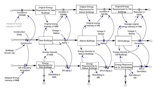
Figure 3: Stock-and-flow-diagram of the building sector
