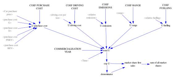
Figure 9 – Structure of the module "Technology Choice" Source: own work using Vensim®
