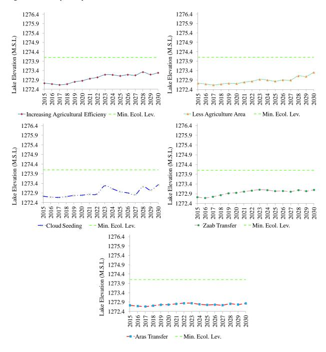
Fig. 7 Simulation of the individual effect of each plan by Urmia SD model
