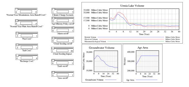
Fig. 6 "Control panel" provided by SyntheSim: Visual and dynamic representation of the Urmia Lake volume affected by changes in the policies and parameters
