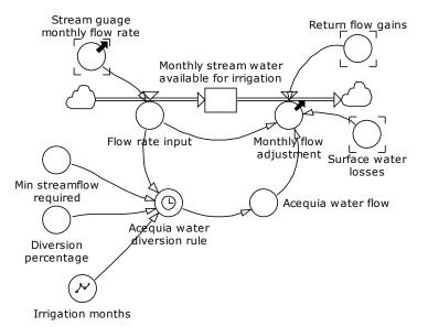
Figure 11. Acequia hydrology stock-flow, with feedbacks for return flow gains and surface water losses.
