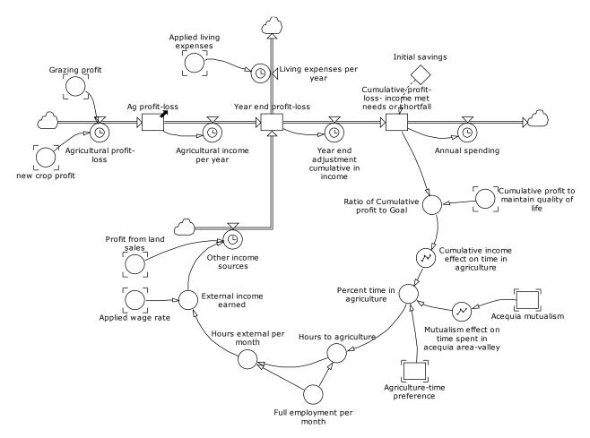
Figure 7. Parciante time management stock-flow structure with associated feedbacks. Each year, agricultural profit and external income are aggregated into Year-end profit-loss. At end of year, this value adjusts the parciate Cumulative profit-loss, which influences Percent time in agriculture for the next year, along with Agriculture-time priority and Acequia mutualism.
