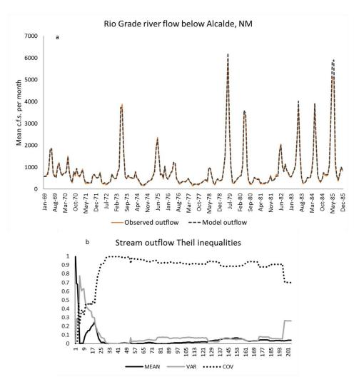
Figure 16. Model reference mode comparison using San Juan Pueblo USGS gauge data (below Alcalde, NM) and model hydrological outflows.
