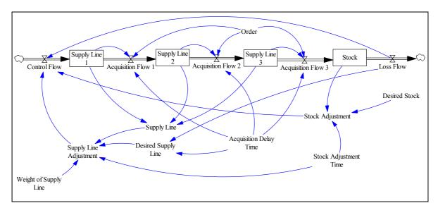
Figure B.36 Stock-flow diagram of the stock management structure with a third order supply line delay
