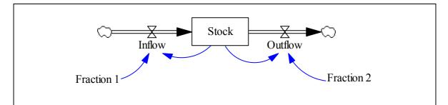
Figure B.5 Stock-flow diagram of the first order linear structure
