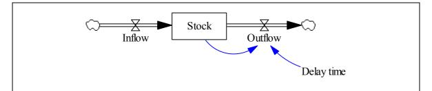
Figure B.16 Stock-flow diagram of the first order continuous material delay structure
