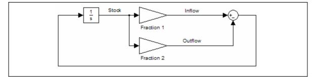
Figure B.6 Block diagram of the first order linear structure
