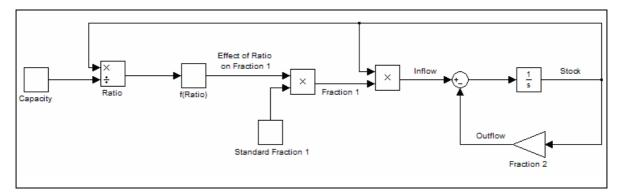
Figure B.12 Block diagram of the capacitated growth structure
