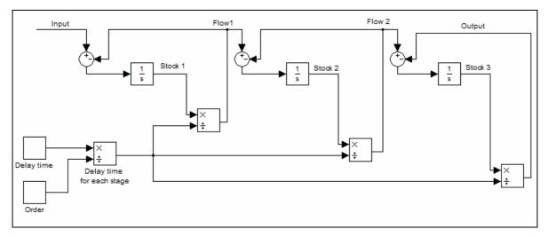
Figure B.19 Block diagram of the third order continuous material delay structure
