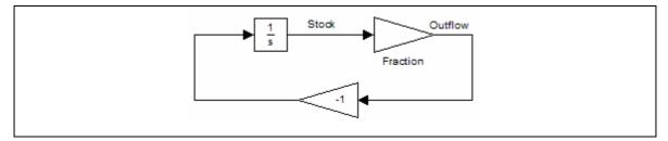
Figure B.4 Block diagram of the draining structure
