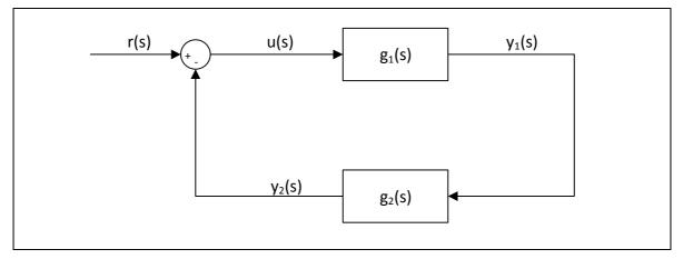
Figure A.2 A block diagram with two blocks
