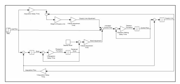
Figure 4. Block diagram of the stock management structure with third order delay
