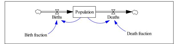
Figure 1. Stock-flow diagram of a basic population model
