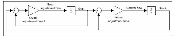
Figure B.31 Block diagram of the simple goal setting structure
