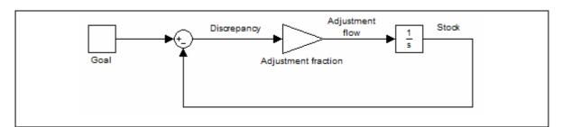
Figure B.10 Block diagram of the goal seeking structure
