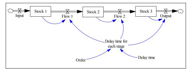
Figure B.18 Stock-flow diagram of the third order continuous material delay structure
