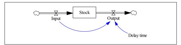
Figure B.24 Stock-flow diagram of the discrete material delay structure
