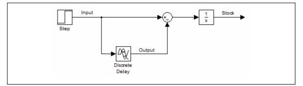
Figure B.25 Block diagram of the discrete material delay structure
