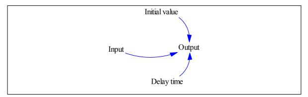
Stock-flow diagram of a discrete information delay structure is given in Figure B.26.
