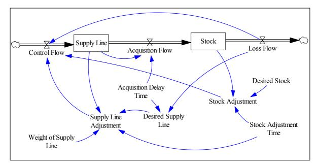
Figure B.34 Stock-flow diagram of the stock management structure with a first order supply line delay
