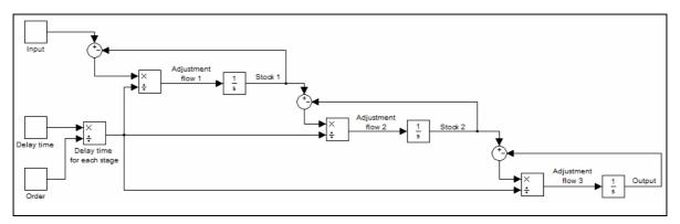
Figure B.23 Block diagram of the third order continuous information delay structure
