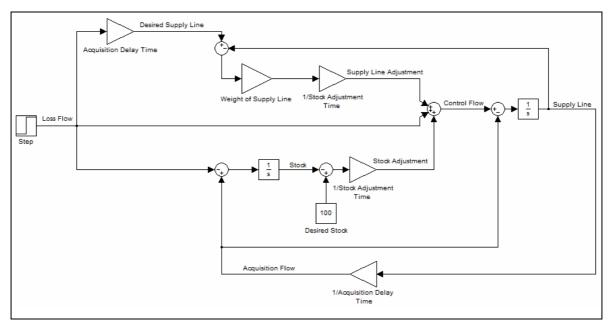
Figure B.35 Block diagram of the stock management structure with a first order supply
