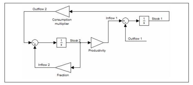
Figure B.29 Block diagram of the oscillating structure
