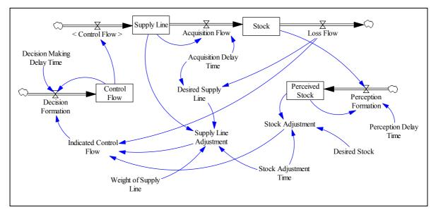
Figure 3. Stock-flow diagram of a stock management structure with three different delay structures
