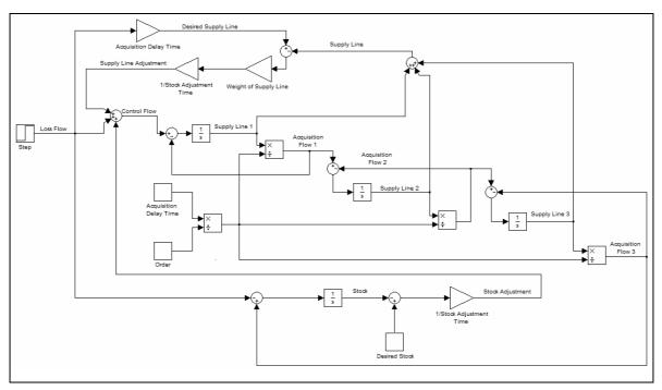
Figure B.37 Stock-flow diagram of the stock management structure with a third order supply line delay
