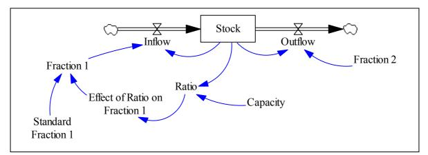
Stock-flow diagram of a capacitated growth structure is given in Figure B.11.
