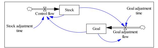
Figure B.30 Stock-flow diagram of the simple goal setting structure
