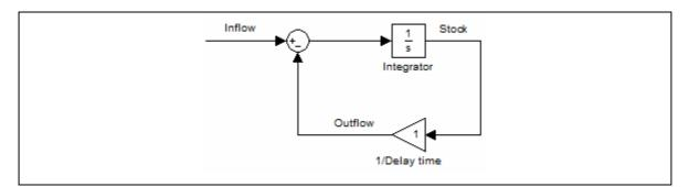
Figure B.17 Block diagram of the first order continuous material delay structure
