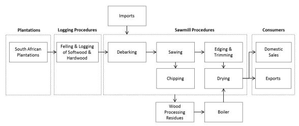
Figure 3: System architecture map for the sawlogs product stream
