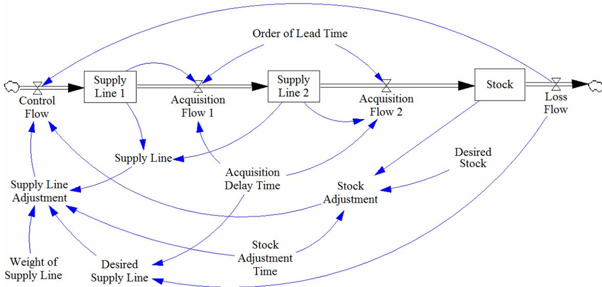
Figure 3. Stock-flow diagram of the stock management task with a 2<sup>nd</sup> order lead time
