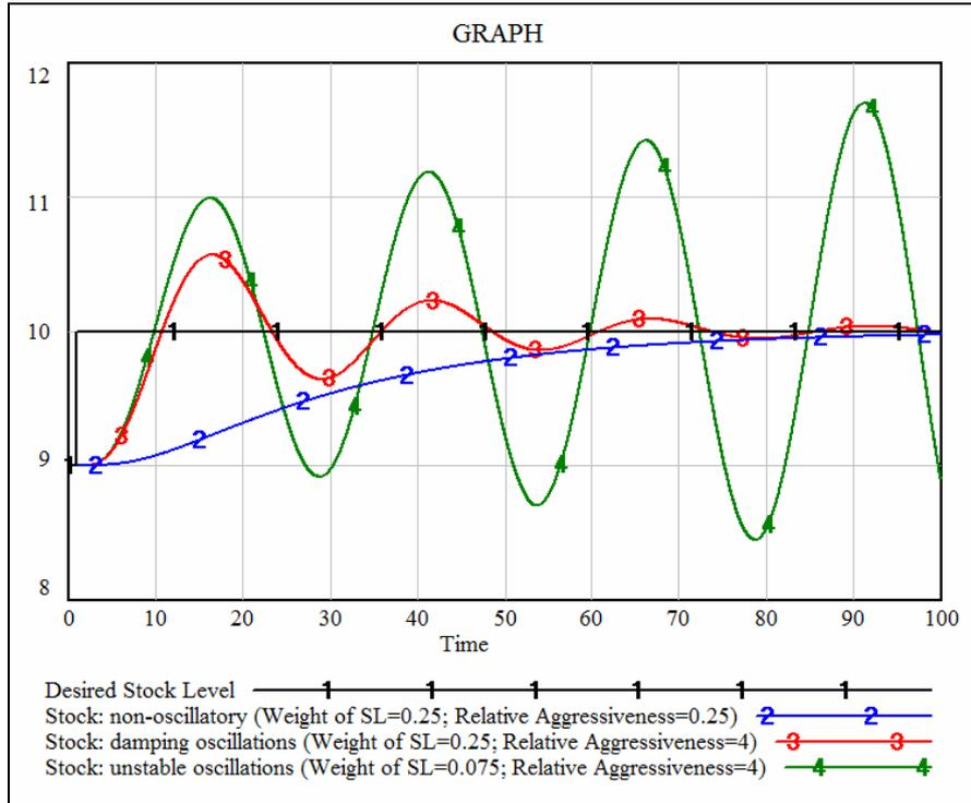
Figure 4. Stock dynamics for different sets of decision parameters
