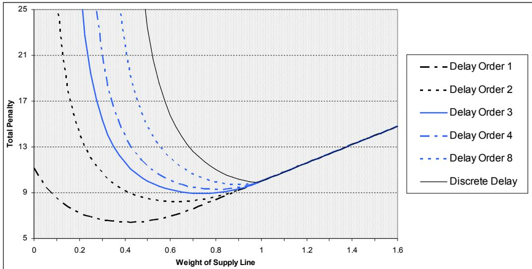
Figure 6. *Total Penalty* plotted against *Weight of Supply Line* when *Relative Aggressiveness* = 4
