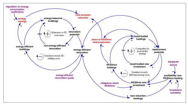
Figure 2: Causal loop diagram of the System Dynamics model
