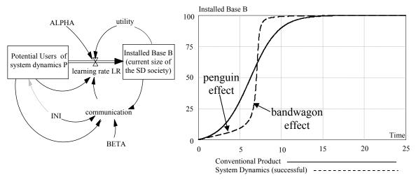
Figure 2: System dynamics diffusion model with network externalities
