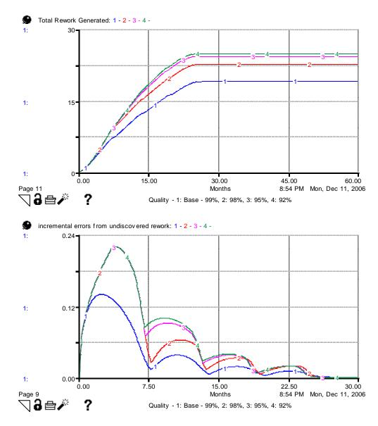
It is interesting to note that giving original work priority in the waterfall case is extremely deleterious to the project's completion (shown below – curve one is the waterfall base case with uncertain requirements, curve two gives priority to original work, and curve three gives priority to rework). Note also that giving priority to rework does not help as much as might have been anticipated (the no priority algorithm in place tends to already favor rework a bit).
